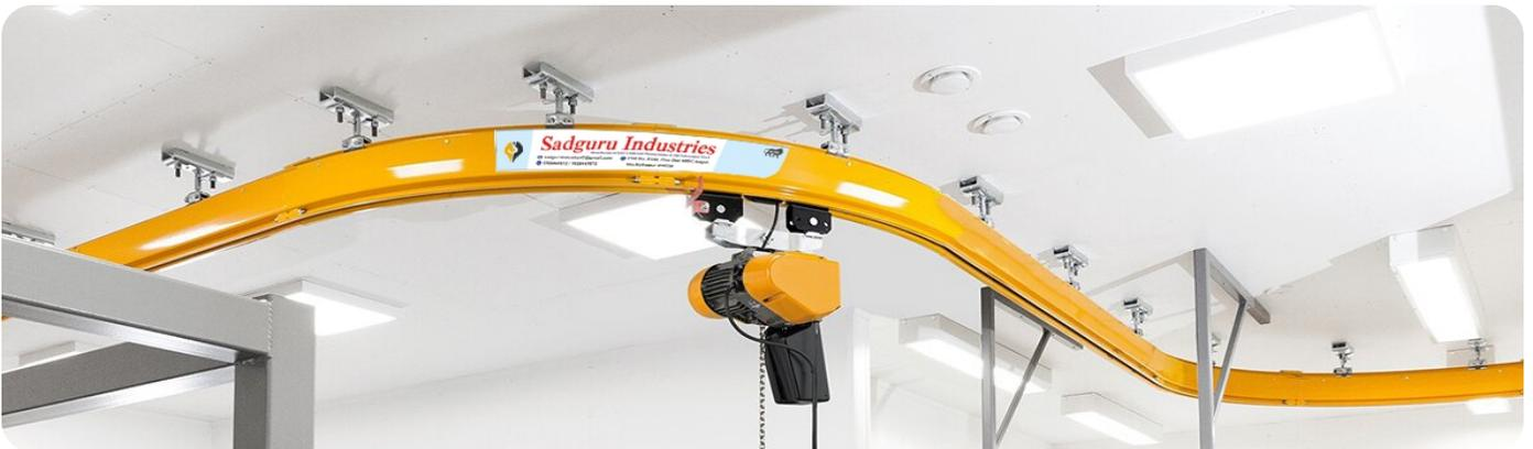
A **Monorail Cranes** Consist Of A Single Rail Or Track System Along Which The Hoist And Trolley Move. This Design Allows For Smooth And Precise Movement Of Loads, Optimizing Material Handling Processes. The Compact And Space-saving Nature Of Monorail Systems Makes Them Ideal For Applications Where Floor Space Is Limited Or Where A Specific Path Of Travel Is Required. One Of The Key Advantages Of Monorail Systems Is Their Adaptability To Individual Applications.
