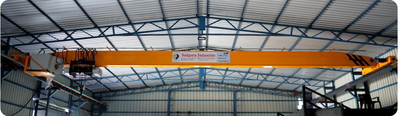
A **Single Girder EOT Crane** Is A Crane That Is Designed For Light And Medium Duty Material Handling. They Are Used For Short Period Work And Light Duty Weight. They Are Ideal For Facilities And Operations With Limited Floor And Overhead Space.
