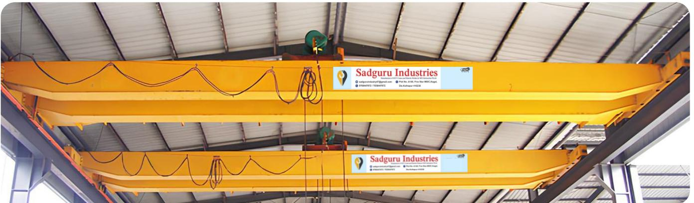
A **Double Girder EOT Cranes** Are A Type Of Electric Overhead Crane That Are Used For Heavy-duty Applications. They Are Made Up Of Two Torsion Free Box Girders.
